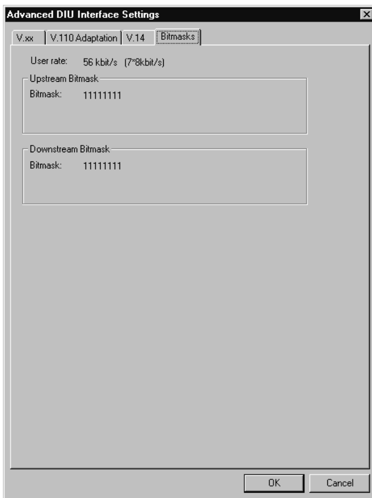
Figure C-12 Bitmasks tab when the intermediate rate is 64 kbit/s or higher
