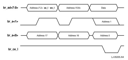
Figure 7–3 Boot ROM Byte Write Cycle
