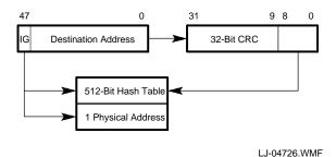
The 21143 can store 512 bits serving as hash bucket heads, and one physical 48-bit Ethernet address. Incoming frames with multicast destination addresses are subjected to imperfect filtering. Frames with physical destination addresses are checked against the single physical address.
