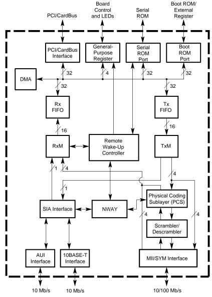
Figure 8-1 21143 Remote Wake-Up Controller Block Diagram
