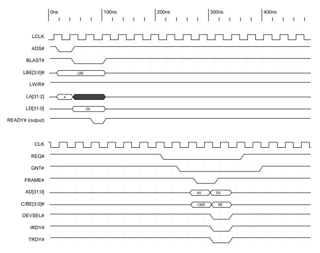
Timing Diagram 5-2. PCI Initiator Single Write
