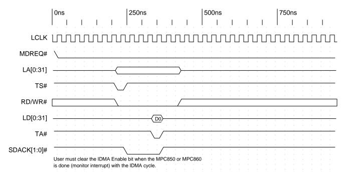
Timing Diagram 3-48. IDMA Single Write Cycle
