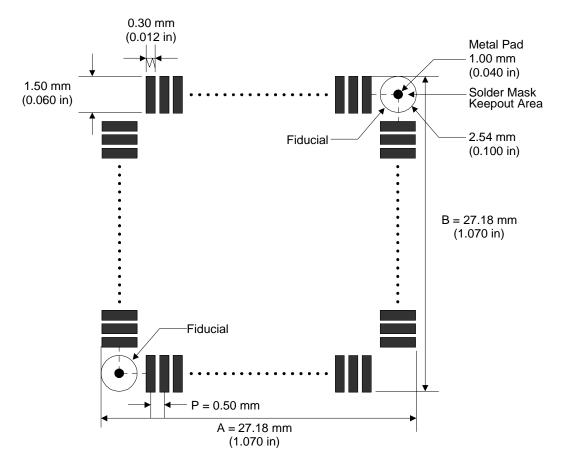
**Note:** Leave 0.002 inch solder mask clearance around pads.
