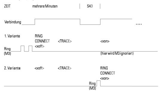
If method 1 is used, the modem first displays the password and phone number of the remote modem after a RING. Then the messages +RNO CARRIER and +RCONNECT (at the time of <xon>) appear as trace text as well as the entries of the remote modem (user password and phone number).
